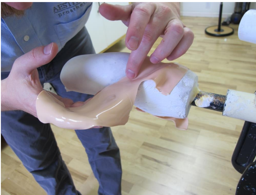
Figure 2. High Consistency Rubber is clay like and can be laid up in sheets.
