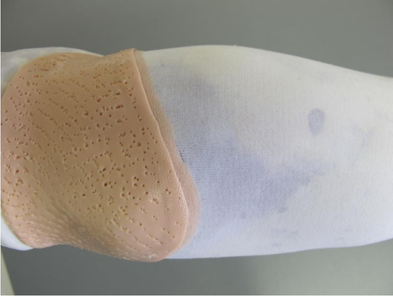
Figure 5. The second layer of silicone before subjecting it to vacuum
