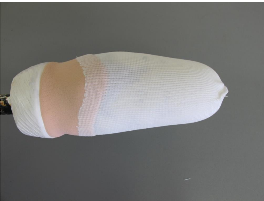
Figure 6. Spectra fabric half embedded
